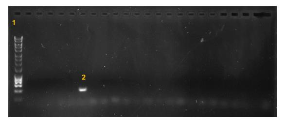
Figure 8. Example of a PCR-positive product in the electrophoresis gel, visualized under UV light. Visualization and image captured using ImageQuant<sup>™</sup> 300 system; GE Healthcare®.
