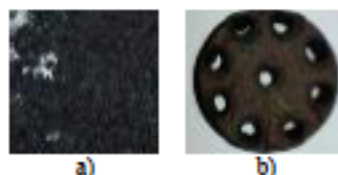
Figure 1. Typical appearance of ACs prepared from MDF precursor in different physical forms (a) powder b) monolith).
