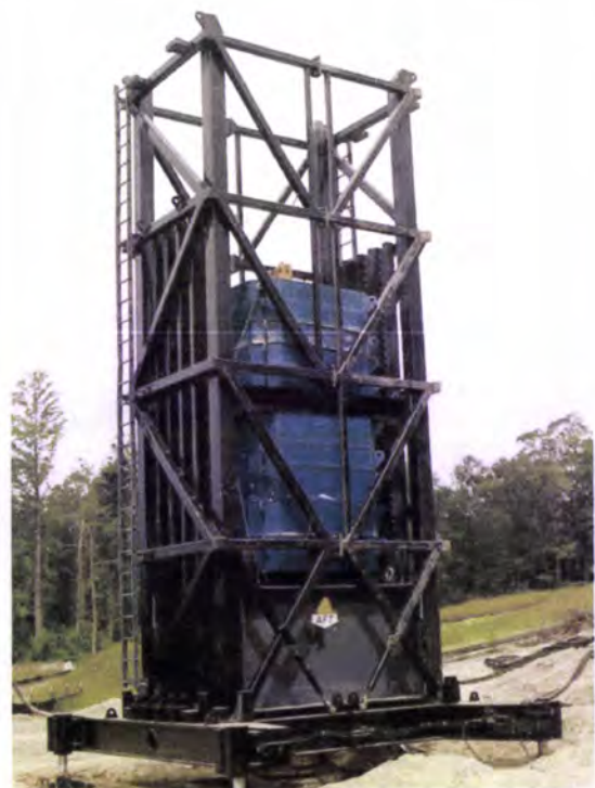
Figure 3 Statnamic Rapid Load Test Device
