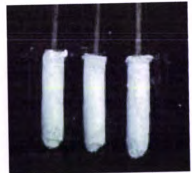
Above: Three model bored piles from the U of Houston Study poured after 24 hrs. of excavation open time show perfect geometry.
