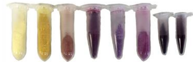
Figure 9: Prepared Lake Pigments. L-R, Weld, Buckthorn, Madder, Brazilwood, Cochineal 1, 2, 3A, and 3B
