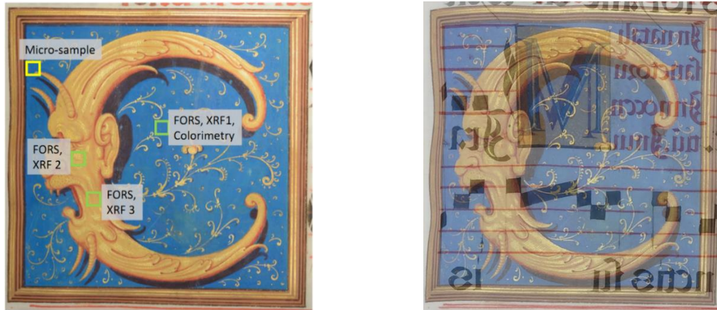
Figure AP II.1: Left, analysis map of f.7r . Right, superimposed recto and verso.
