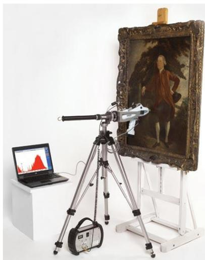
**FIGURE 8. EXAMPLE OF PORTABLE XRF WITH VACUUM PUMP, TRIPOD AND COMPUTER FOR DATA ANALYSIS (IMAGE TAKEN FROM [HTTP://GOO.GL/KKZRVX](http://goo.gl/kkzrvx))**
