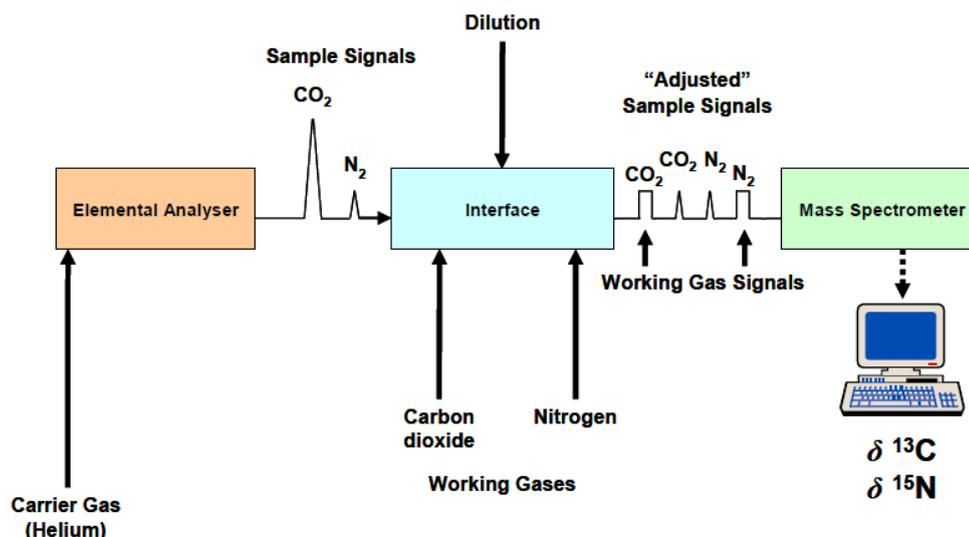
Figure 14 Simplified schematic drawing of an EA-IRMS setup for the determination of  $\delta^{13}\text{C}$  and  $\delta^{15}\text{N}$ , taken from (Carter, et al., 2011), p. 3.
