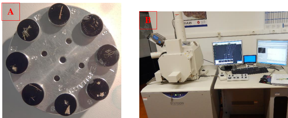
Figure 47 a) Samples mounted in carbon coat for VSEM-EDS analyses b) VSEM-EDS instrument used in the study of the Francisco Pizarro's Banner
