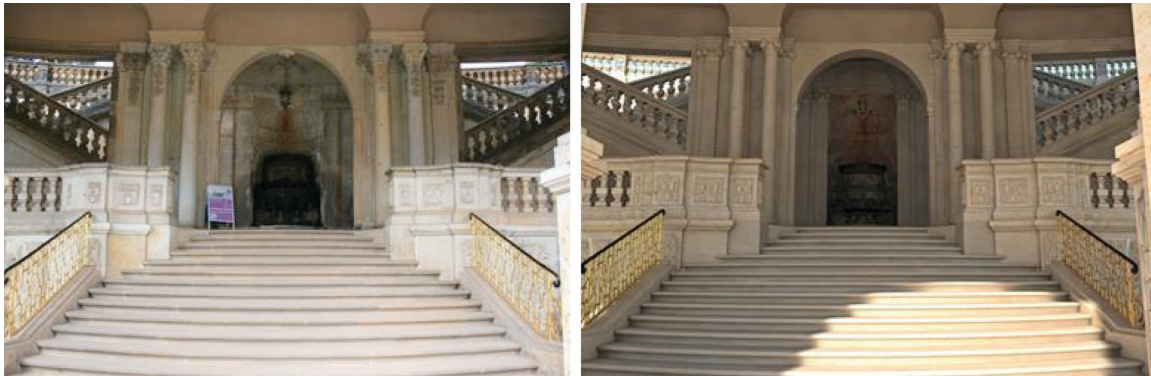
Fig. 18 Inner staircase of the western central pavilion (so-called Wallpavillon) of the Dresden Zwinger Left: photograph of the original building from 2012 Right: rendering of a textured polygon model from 2012 (software: Cinema 4D).
