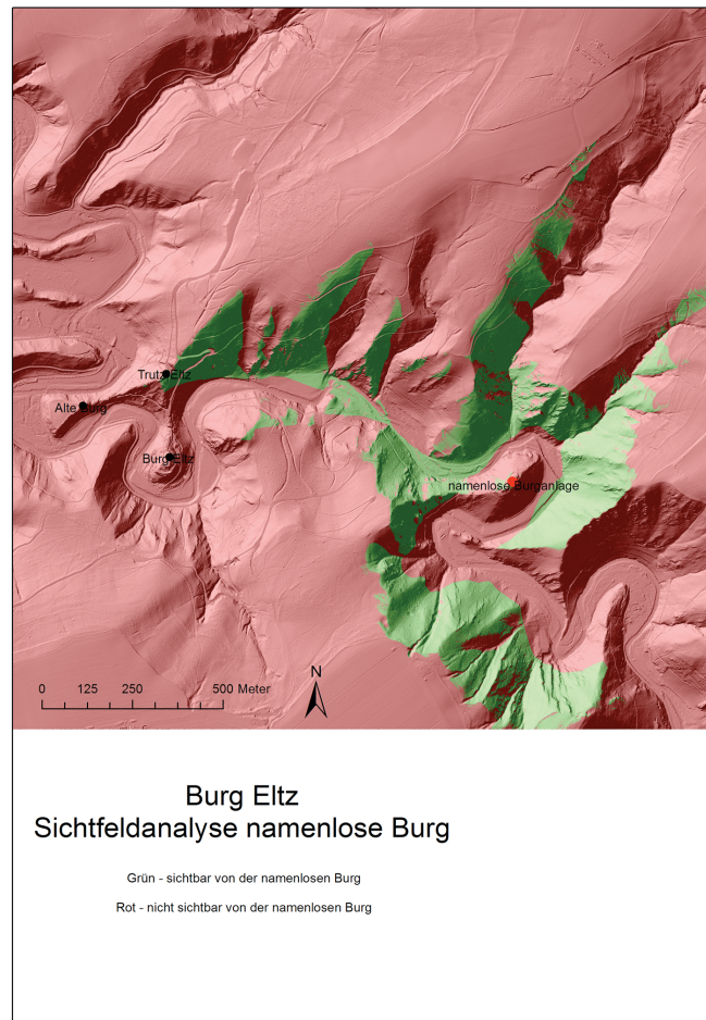
Fig. 14 Castle Eltz, LiDAR-scan, green are the areas that can be seen from a person standing on the nameless castle (2010).
