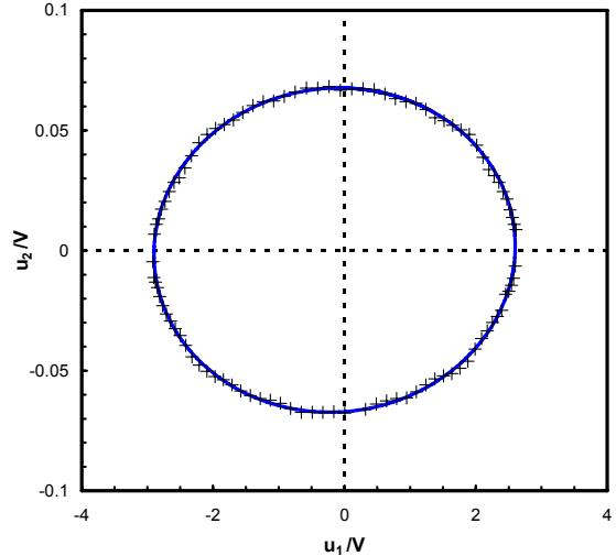
Fig. 12. Sampled points and the fitted ellipse.  $u_1$  corresponds to the function generator voltage while  $u_2$  is the voltage across a  $200 \Omega$  resistor which is connected in series with a  $20 \text{ nF}$  capacitor.
