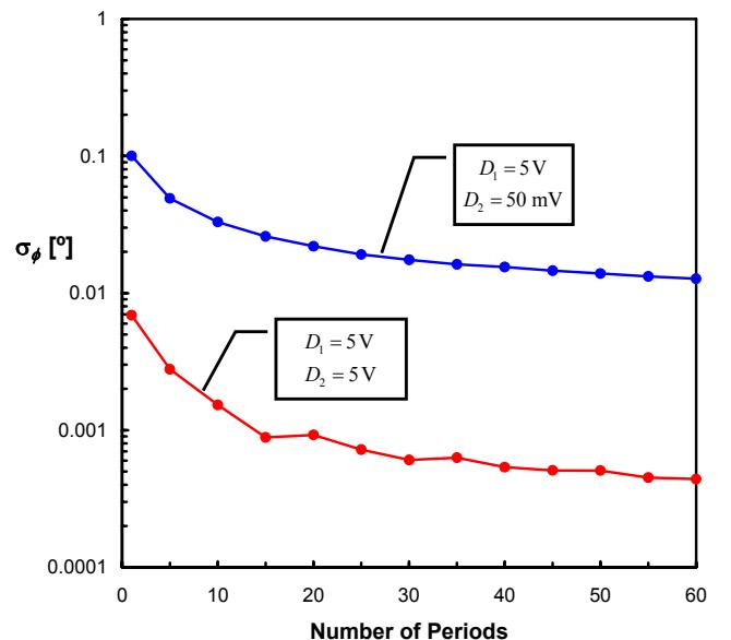
**Fig. 10.** Standard deviation of the phase error as a function of the number of acquired periods for two different amplitude combinations.
