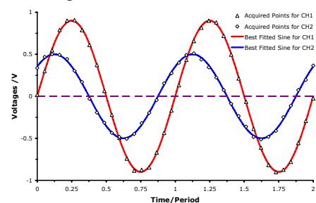
**Fig. 1. Time-domain fitting of two acquired noisy sine signals with common frequency and  $f_s/f = 18.5$ .**
