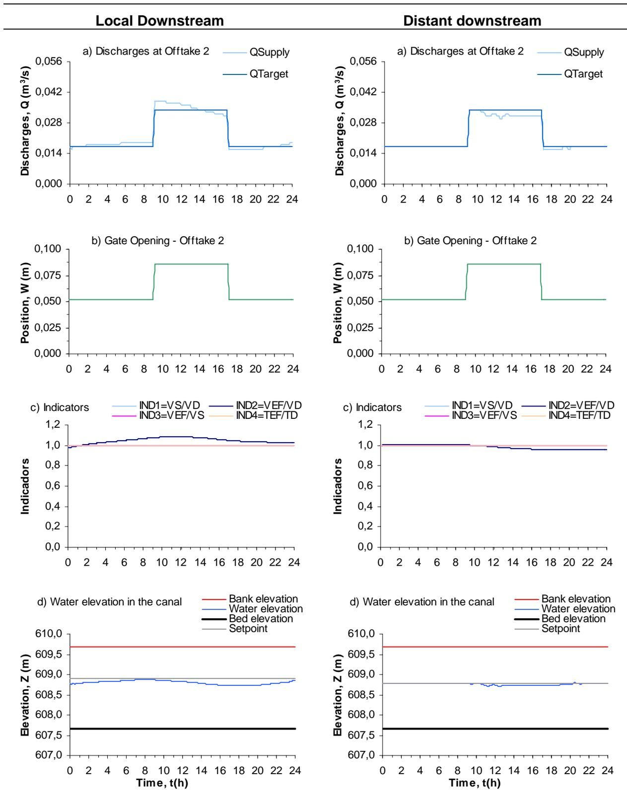
Figure 4. Hydraulics simulation results for the Offtake 2, considering all the offtakes as gate controlled weirs.
