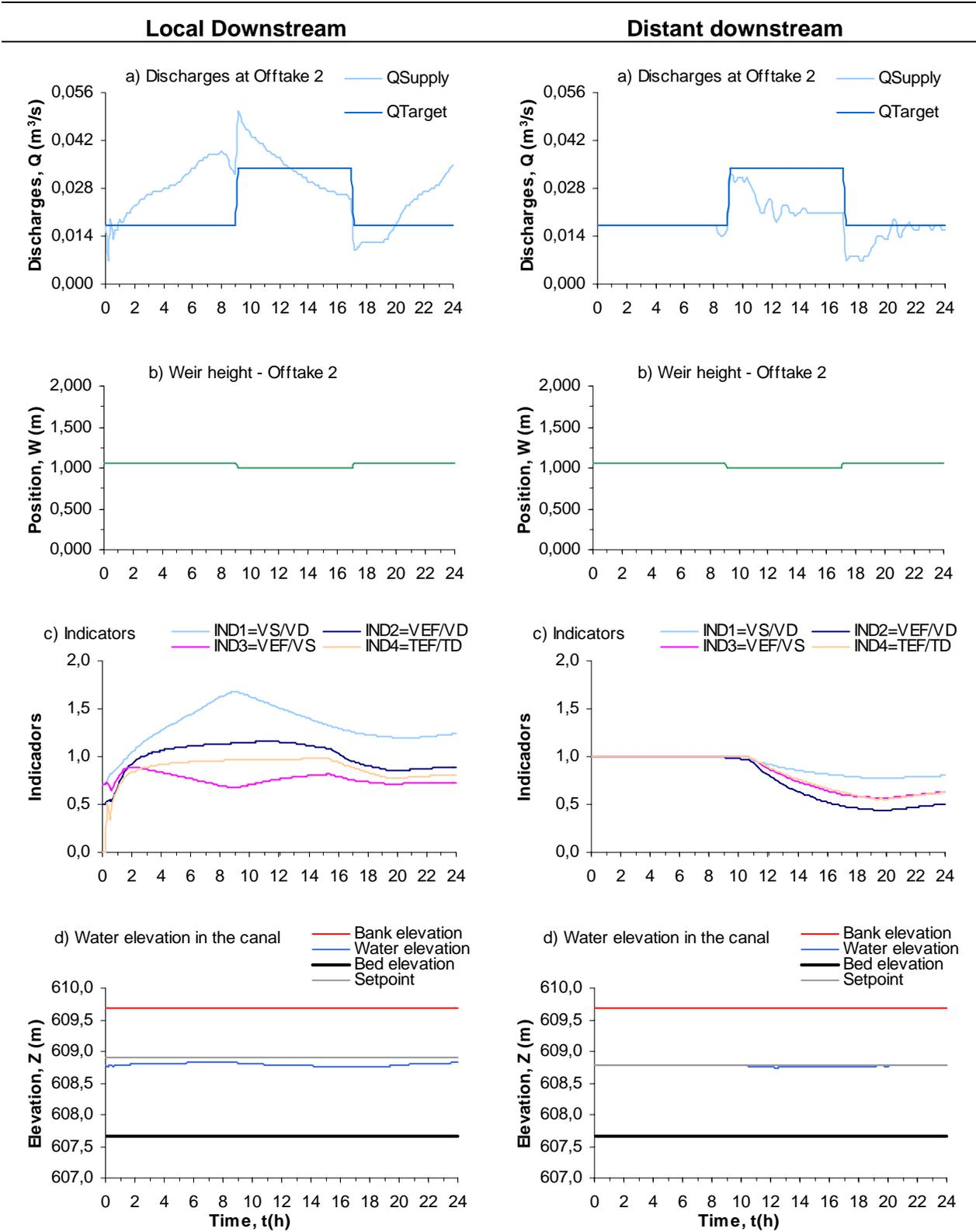
Figure 6. Hydraulics simulation results for the Offtake 2, considering all the offtakes as weirs with adjustable heights.
