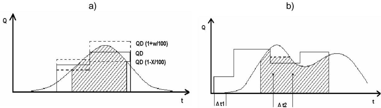
Figure 3. Definition of the effective volume (a) and time indicator (b).
