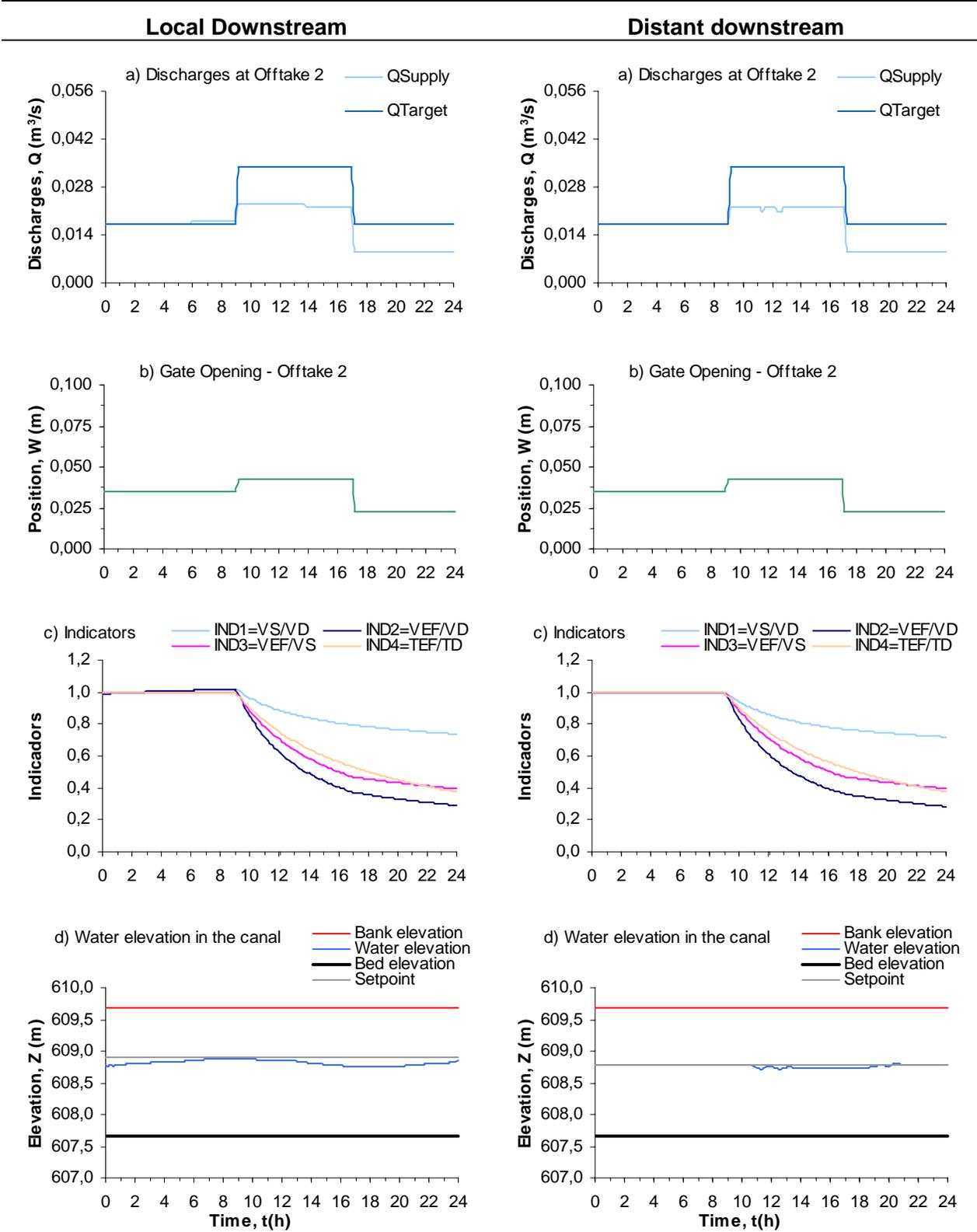
Figure 5. Hydraulics simulation results for the Offtake 2, considering all the offtakes as gate controlled orifices.
