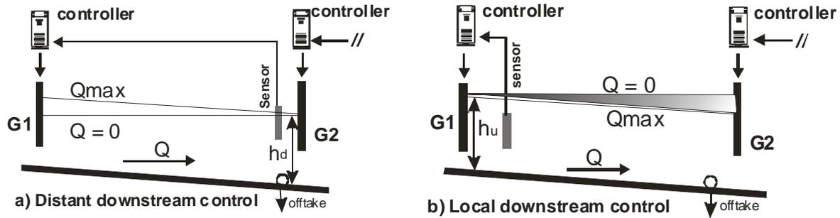
Figure 1. Distant and local downstream canal control modes.
