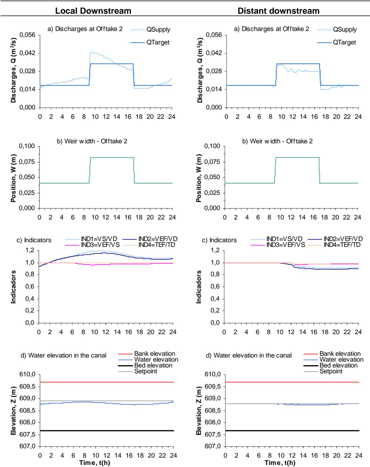
Figure 7. Hydraulics simulation results for the Offtake 2, considering all the offtakes as Weirs without adjustable heights (variable widths).
