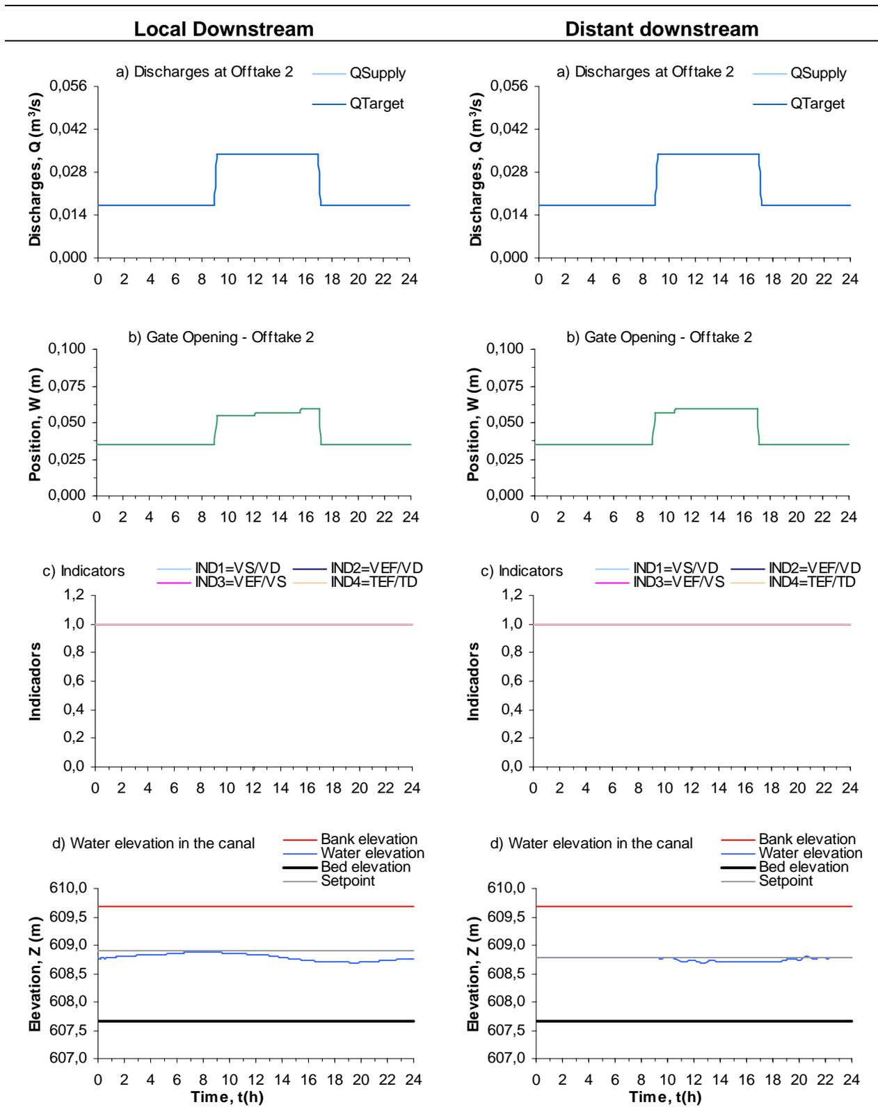
Figure 8. Hydraulics simulation results for the Offtake 2, considering all the offtakes as automatic flow adjustable offtakes (gate controlled orifices).
