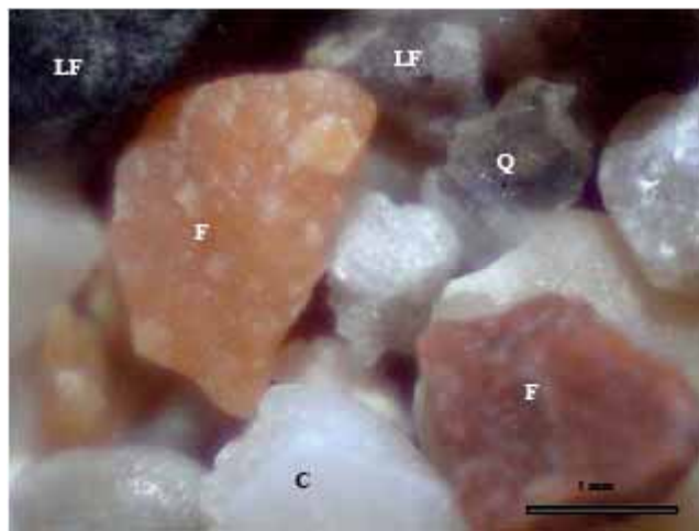
Fig. (2). Verona (Binocular OM image). Sand grains of reddish Feldspars (F), Quartz (Q), Calcite (C) and volcanic lithic fragments (LF).
