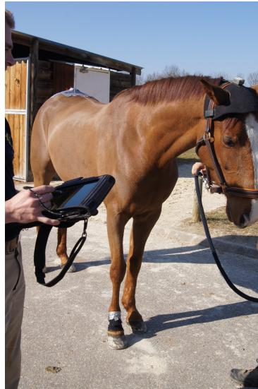
Figure 1: Horse instrumented with 3 inertial sensors during a lameness exam. There is a uni-axial accelerometer attached to the head bumper; one uni-axial accelerometer placed between the tubera sacrale on the midline of the most dorsal aspect of the pelvis with tape and a third uni-axial gyroscope wrapped to the dorsal aspect of the right forelimb pastern (VetAgro Sup - Veterinary Campus of Lyon).
