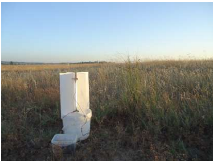
Figure 2: Light trap used to capture arthropods during this study.
