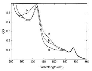
Fig. 1. UV-visible spectra of ROO in several redox states. *Trace a,* as prepared ROO  $(1.5~\mu\text{M})$  in 50 mM Tris-HCl buffer, pH 7.6; *traces b* and c, partially reduced samples with dithionite. Only 3 out of 46 spectra from a titration in the absence of redox mediators are shown.
