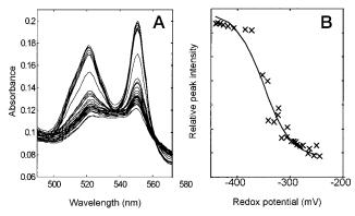
FIG. 5. **Visible redox titration of ROO hemes.** Panel A, visible spectra of ROO obtained along the redox titration varying the potential from -250 to -449 mV. Panel B, titration curve of ROO hemes followed at 550 nm, corrected in respect to 565 and 535 nm isosbestic points. The line corresponds to a Nernstian process,  $E_m = -350$  mV, n = 1.
