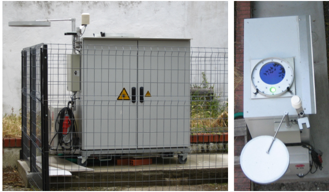
Figure 2.1.: PAOLI with open roof cover from the front (left) and from the top (right).
