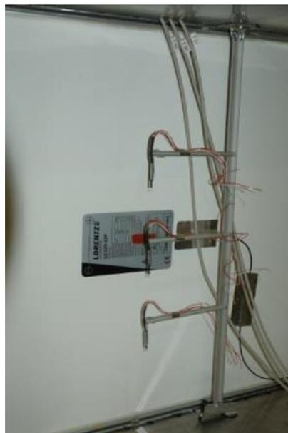
Fig. 5.5. Detail of the support structure for the three air temperature sensors
