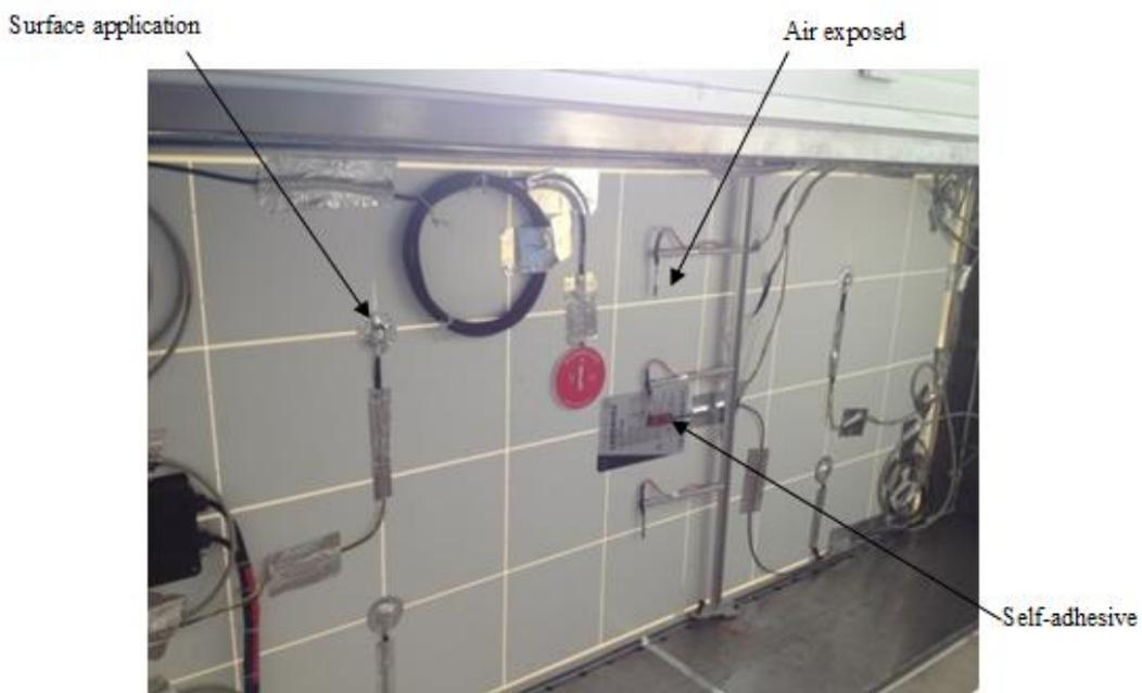
Fig. 5.8. PT 100 sensor (a), PT 100 Self-adhesive sensor (b)
