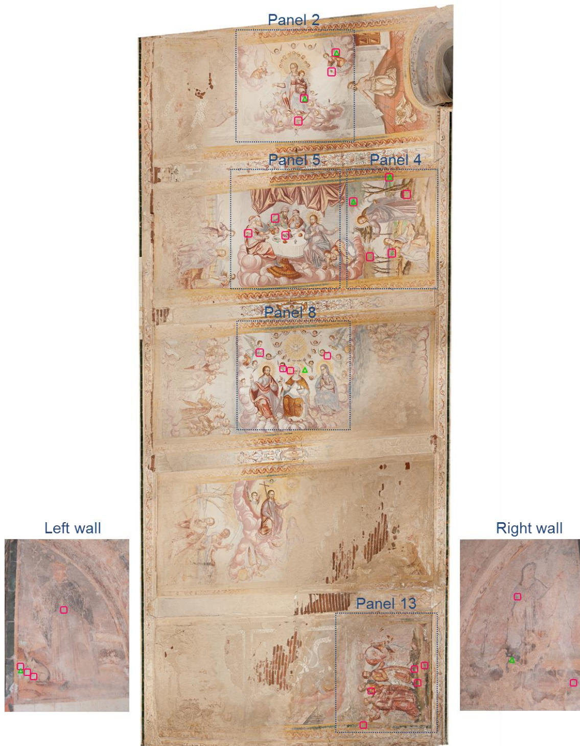
Figure II-13. Sampling location on green, brown and golden areas of the panels 2, 4, 5, 8, 13, and from Left and Right wall (□ - samples collected with sterile cotton swabs; ▲ - microfragments collected with sterile scalpels and microtubes) present in the Low Choir of the Convent of Nossa Senhora da Saudação Church, Montemor-o-Novo, Portugal).
