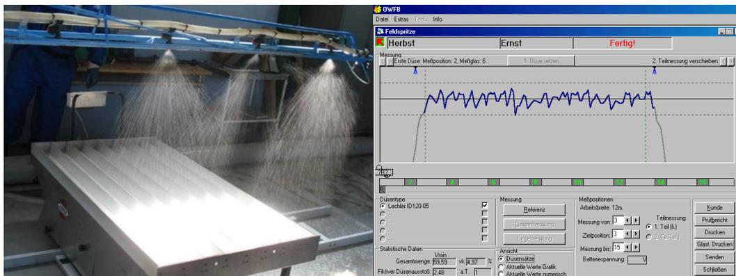
Figure 6.2. The electronic groove table for testing uniformity of distribution of atomized liquid fall and a protocol from these tests
