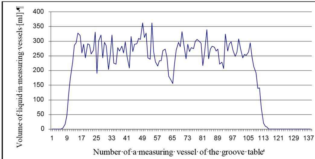
Figure 6.7. Characteristics of nozzle liquid fall obtained on a virtual groove table of grooves 100 mm wide for the sprayer TTD JET RS 110 R with the pressure of 3 bars. CV =15 %
