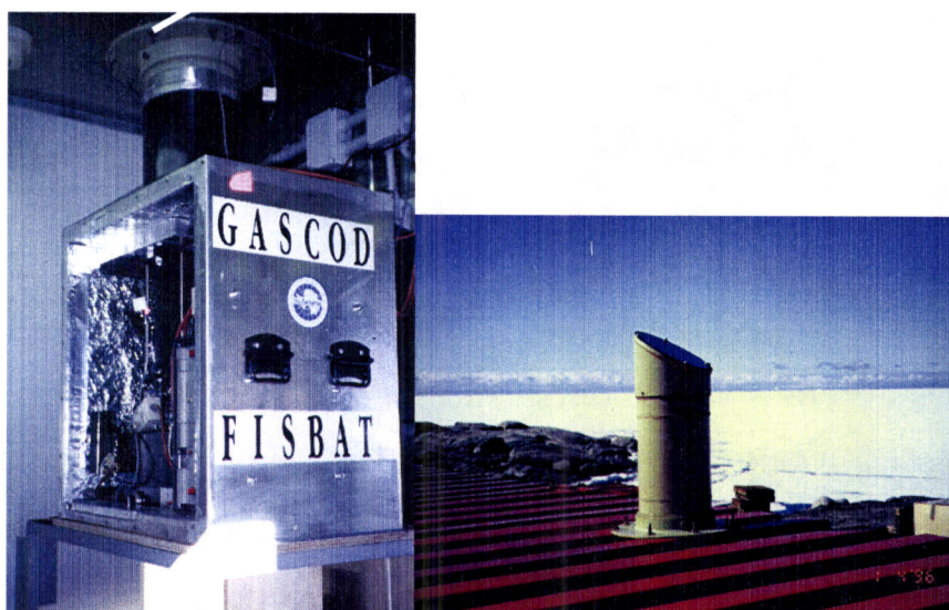
Figure 5.2 – GASCOD Spectrometer installed at the Italian Antarctic Station since 1995 (left), Optical chimney for the input of the radiation(right).
