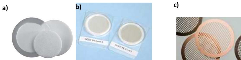
Figura 15 – a) e b) filtros de quartzo; c) TEM grids.
