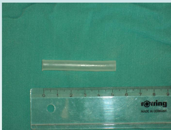
Figure 1- PVA/Dx graft 5 cm length/ 5 mm internal diameter.
