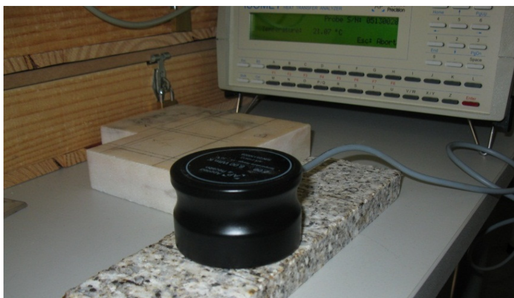
Figure 2 -Heat Tranfer Analyser ISOMET 2104. The measuring probe is the black device on top of the rock sample.
