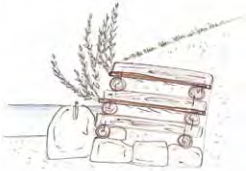
Figure 4.5.5.1 Side view of a vegetated log crib wall (Paola Sangalli)
