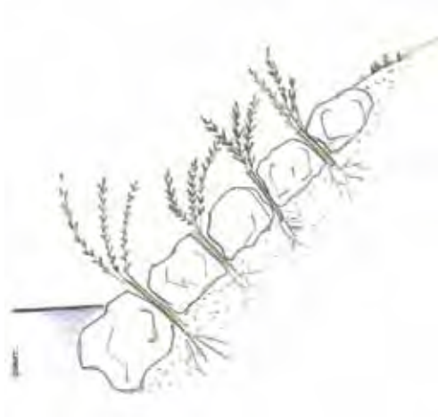
Figure 4.5.2.2 Riprap with live stakes (Paola Sangalli).
