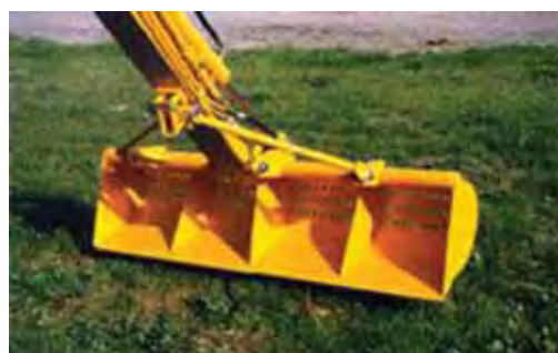
Figure 4.4.2 Perforated shovel that can be used for Water Hyacinth removal (Photo: I. Moreira).
