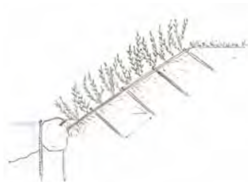
Figure 4.5.4.2 Side view of a brush mattress on a riverbank (Paola Sangalli).
