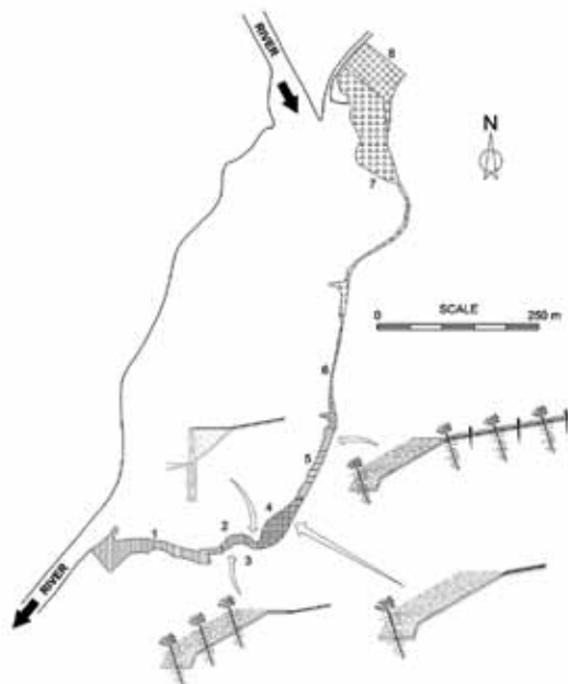
Figure 1.3.8 Examples of the mixed techniques used for rehabilitation along one of the banks of the widened channel of the River Tâmega. From downstream to upstream: 1. rip rap and establishment of sods and grasses; 2. rip rap and joint planting; 3. post wall; 4. toe rip rap and bank shaping covered with grass; 5. toe rip rap and branch mattress (with live stakes); 6 and 7. weed cutting and removal of soil heaps; 8. recreational area.
