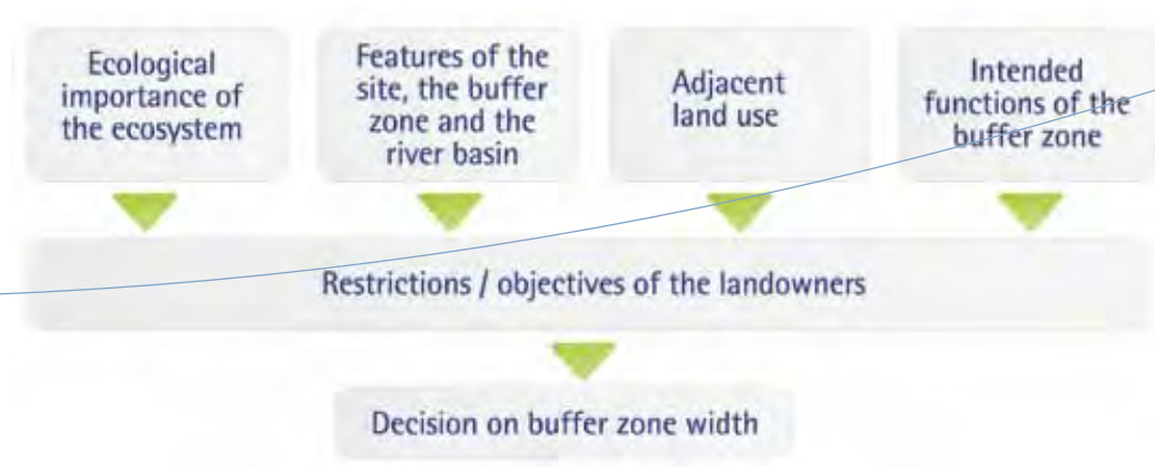
Figure 4.8.1 Criteria for determining the width of a river buffer zone (adapted from Palone and Todd, 1998).
