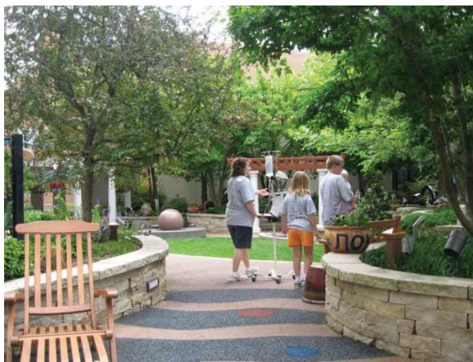
Figure 115 A rubberized walking surface facilitates use of the garden by those using wheelchairs or pulling an IV pole (Marcus & Sachs, 2014).
