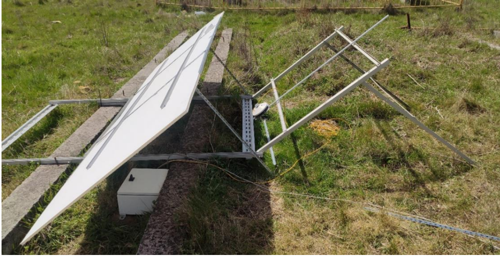
Fig. 4.3 - Experimental setup for measuring global tilt irradiance for different positions.
