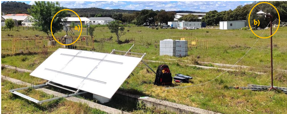
Fig. 4.4 - Overview of the experimental setup including a) the Évora – PECS station and b) the pyranometers used for albedo computations.
