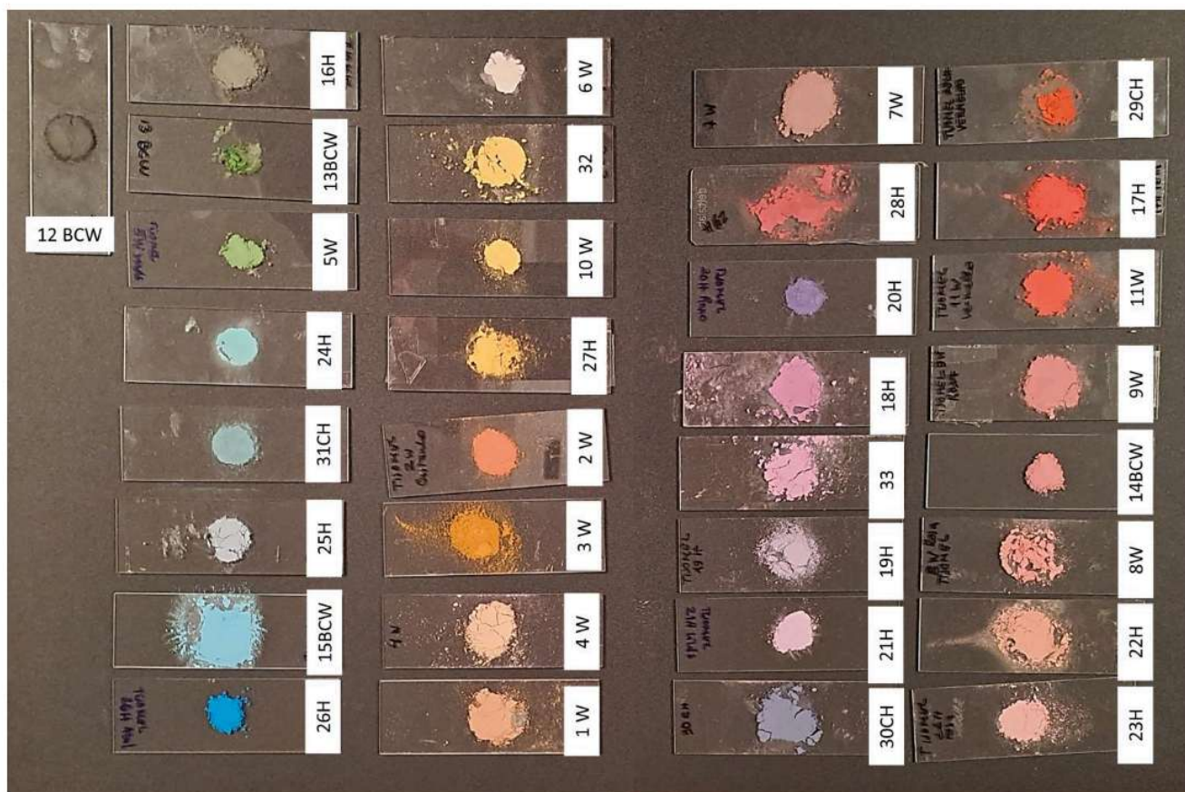
Figure 3. Samples of Tijomel raw materials, colourants and glaze on glass slides (reference according to Table 1).
