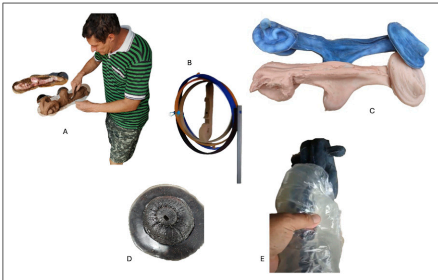
Figure 3. Illustration of the production process of the Nelore cow reproductive tract and rectum models. (A) External modeling of the reproductive device using measurements. (B) Utilization of a gyroscope for silicone rubber distribution. (C) Female reproductive model in various silicone varieties. (D) Anus of the simulator crafted with thermolabile silicone. (E) Bag containing a slime-type solution.
