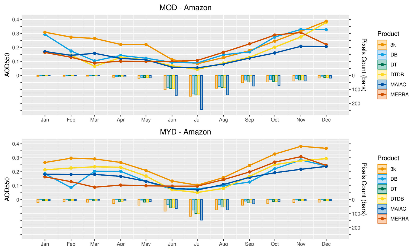
Fig. 11. Seasonal pattern of AOD550 with monthly mean (colored lines), and number of pixels (bars) in the NEB biome domain of Amazon from 2015 to 2018 for Terra (MOD) and Aqua (MYD) satellites products. There are scale factors in the pixels count scale of 10^2 (DT, DB, DTDB), 10^3 (3 k), and 10^4 (MAIAC). (For interpretation of the references to colour in this figure legend, the reader is referred to the web version of this article.)
