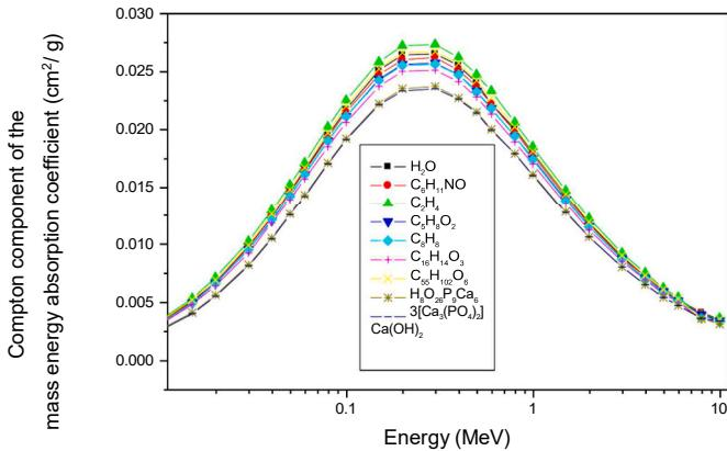
**Fig. 9.** Compton component of mass energy absorption coefficients ( $\text{cm}^2/\text{g}$ ) for few biological materials in the energy region from 0.005 to 10 MeV estimated using mixture rule.
