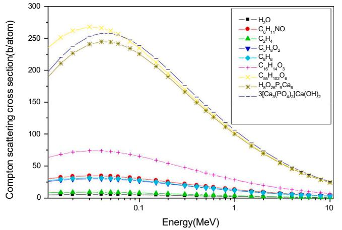
**Fig. 5.** Whole-atom total Compton scattering cross-sections (b/atom) for the biological materials in the energy region from 0.5 to 10 MeV using the tabulated values of XCOM (Berger and Hubbell 1987).
