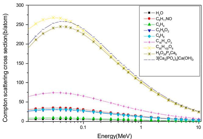
**Fig. 3.** Whole-atom total Compton scattering cross-sections (b/atom) for the biological materials in the energy region from 0.5 to 10 MeV using the tabulated values of Biggs et al., (1975).
