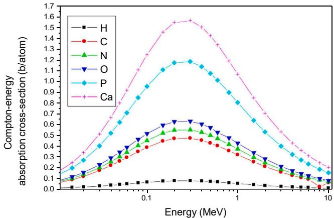
**Fig. 2.** Compton energy absorption cross-sections (b/atom) for H, C, N, O, P and Ca in the energy region 0.005–10 MeV, using the tabulated values of Biggs et al., (1975).
