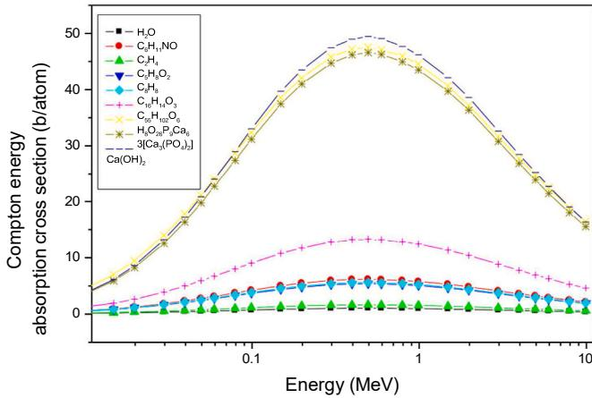
**Fig. 7.** Compton scattering energy absorption cross-sections (b/atom) for the biological materials in the energy region from 0.5 to 10 MeV using the tabulated values of Storm and Israel (1970).
