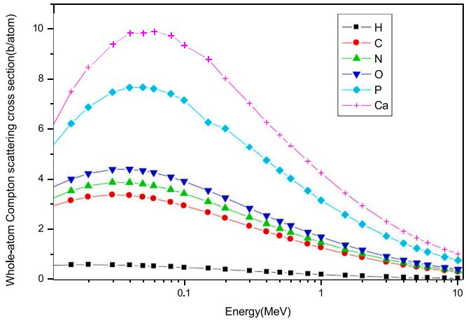
**Fig. 1.** Compton scattering cross-sections (b/atom) for H, C, N, O, P and Ca in the energy region 0.005–10 MeV, using the tabulated values of Biggs et al., (1975).
