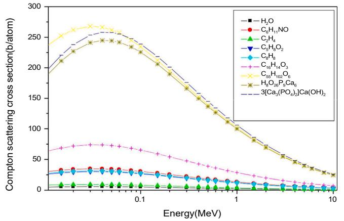
**Fig. 4.** Whole-atom total Compton scattering cross-sections (b/atom) for the biological materials in the energy region from 0.5 to 10 MeV using the tabulated values of Storm and Israel (1970).
