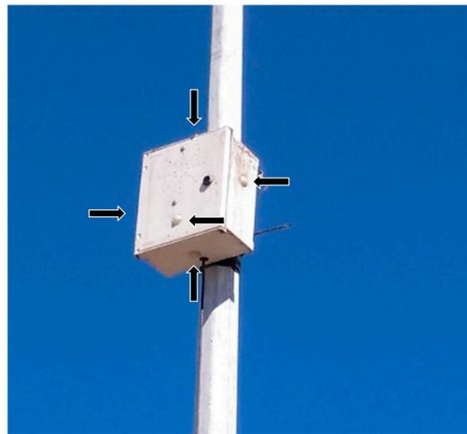
**Figure 1.** Deterrent device with the location of the PIR sensors (indicated by arrows).
