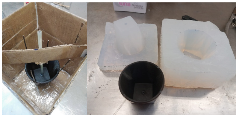
Fig. 6. Fabrication of the mould in order to produce the silicone mould itself.
