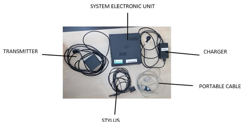
**Fig. 1.** Main parts of Fastrak Polhemus device (electro-magnetic tracking system).
