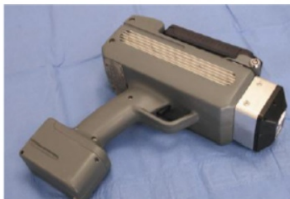
Figure 6: Tracer II Unit- 1st X-ray tube with silver (Ag) anode from key master(2001) (Portable Spectral Service, n.d)
