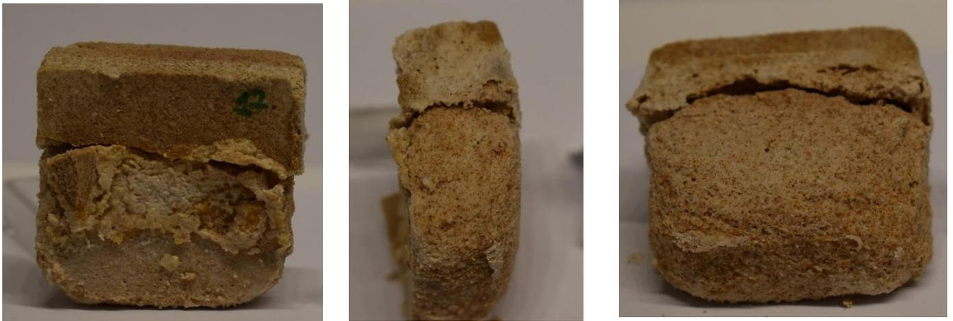
Figure 27: POS-15-HL after the 12th cycle showing a complete disintegration
