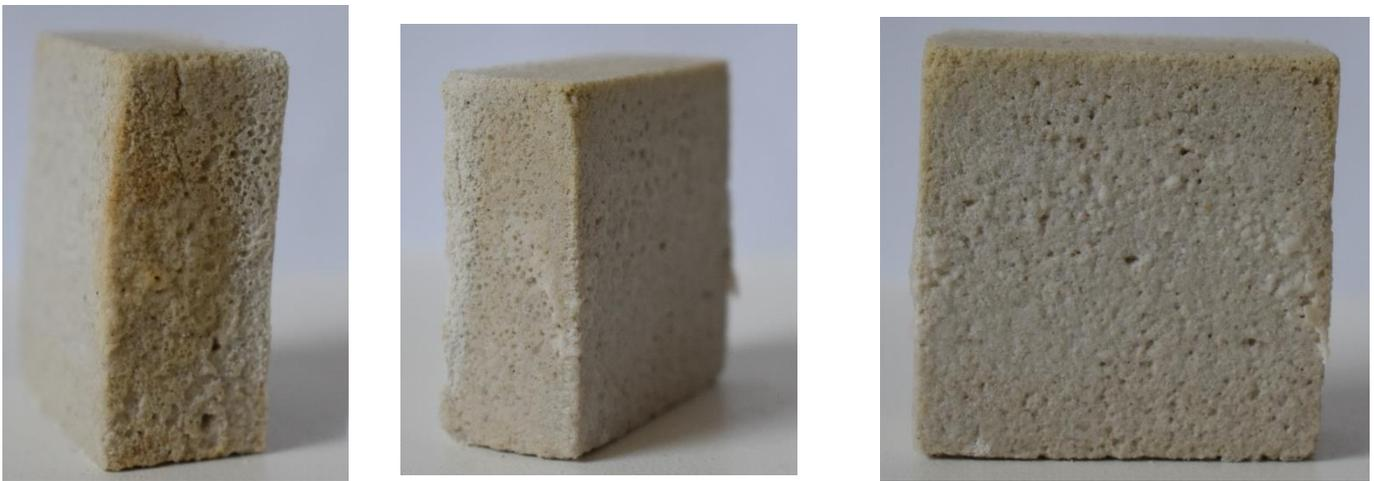
Figure 33: TQ-HL showing early signs of blistering after the 3rd cycle.
