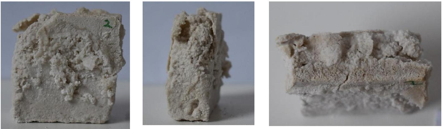
Figure 25: TQ samples after the 15th cycle showing significant material loss at the end of the test
