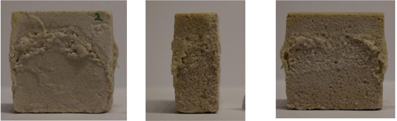
Figure 26: TQ samples after the 10th cycle showing signs of exfoliations
