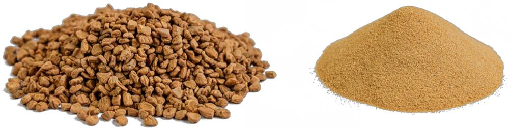
Figure 9: Left- Unmilled olive stones, Right- Ground olive stone (100-300microns). Retrieved from: [www.bio-powder.com/en/olive-pit/](http://www.bio-powder.com/en/olive-pit/)
