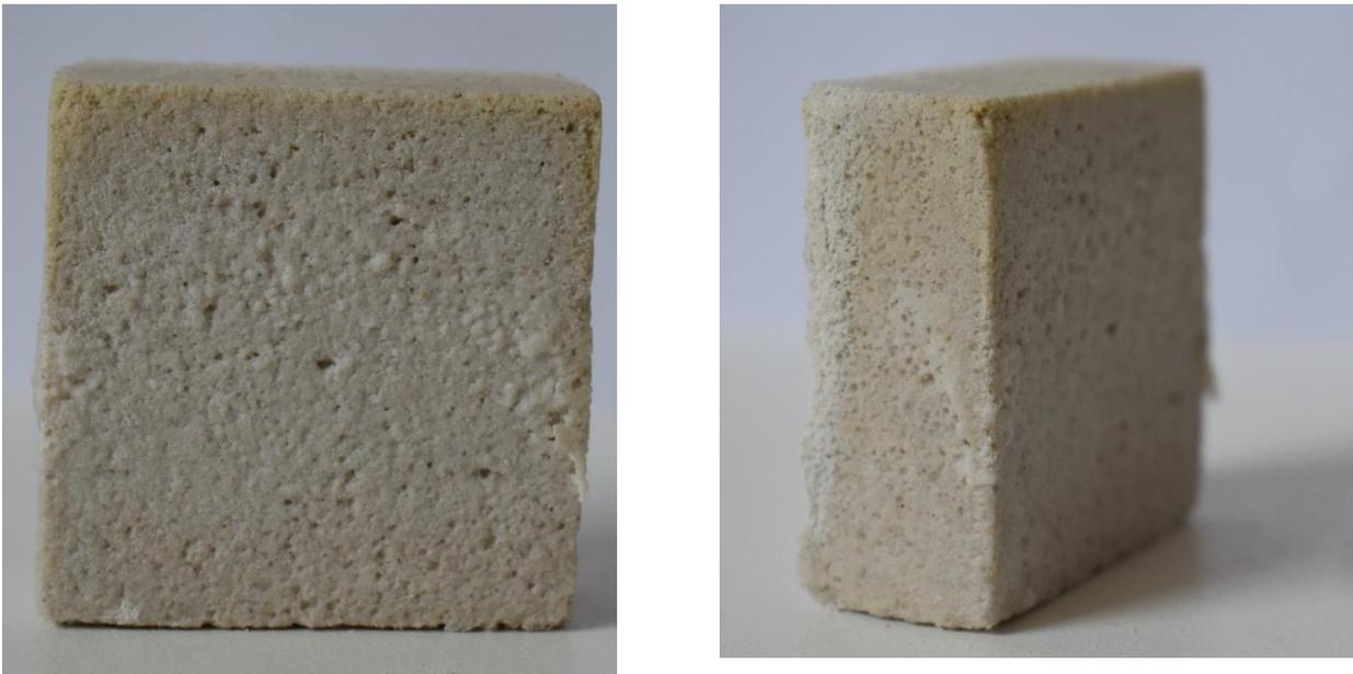
Figure 30: TQ samples showing signs of minor blistering and tiny salt crystals on its surface after the 3<sup>rd</sup> cycle of the salt crystallization cycle
