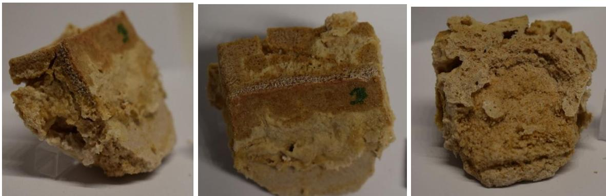
Figure 35: The last sample of POS-10-HL-S disintegrating after the 12th cycle
