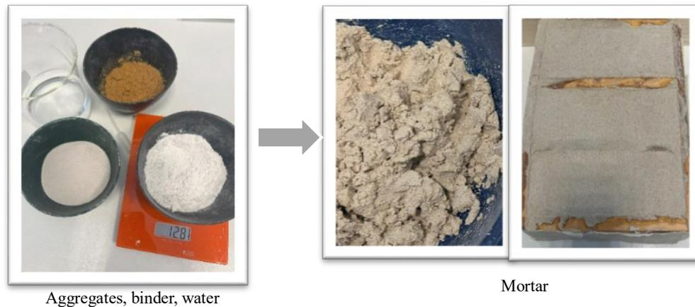
Figure 1: Mortar composition
