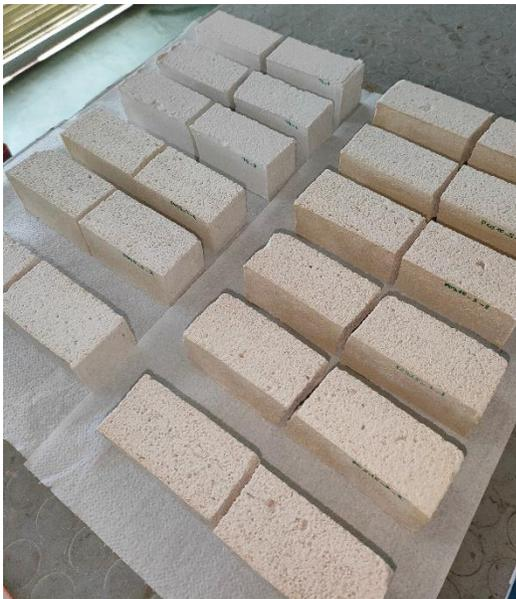
Figure 18: Halved specimens after flexural strength test
