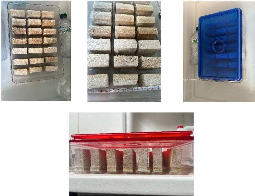
Figure 13: Representation of how the specimen were contaminated with the sodium sulphate solution while maintaining the temperature of the solution in a water bath
