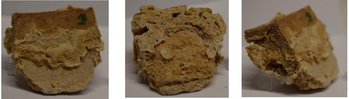
Figure 29: POS-10-HL-S after the 12th cycle completely disintegrated
