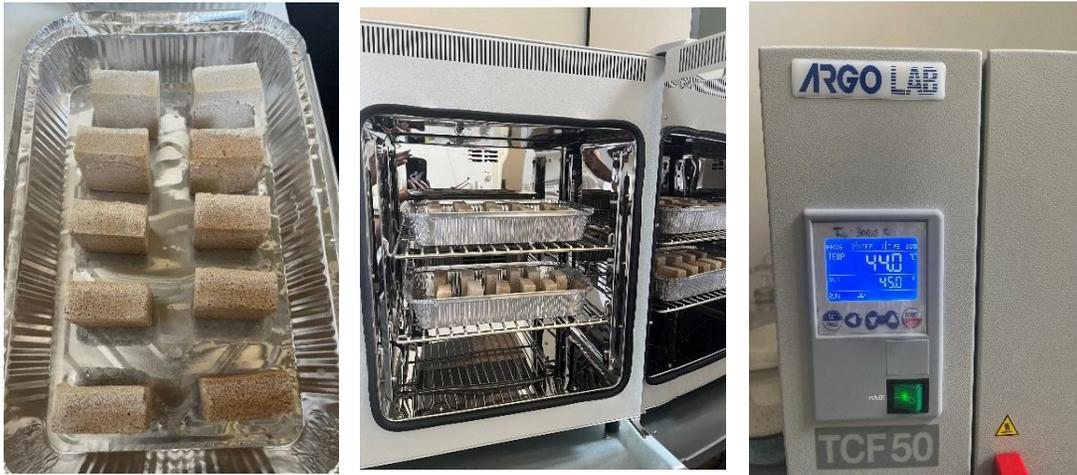
Figure 14: Drying of the specimens after immersion
