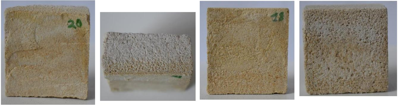
Figure 32: POS-HL-S series showing no signs of suffering the salt weathering test after the 3rd cycle as compared to the TQ-HL below
