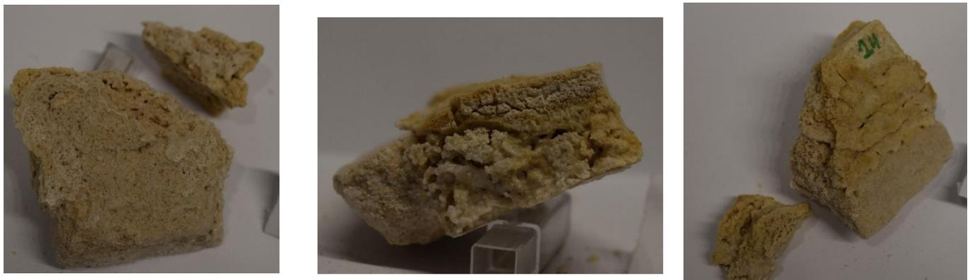
Figure 28: POS-5-HL-S after completely disintegrated after the 14th cycle
