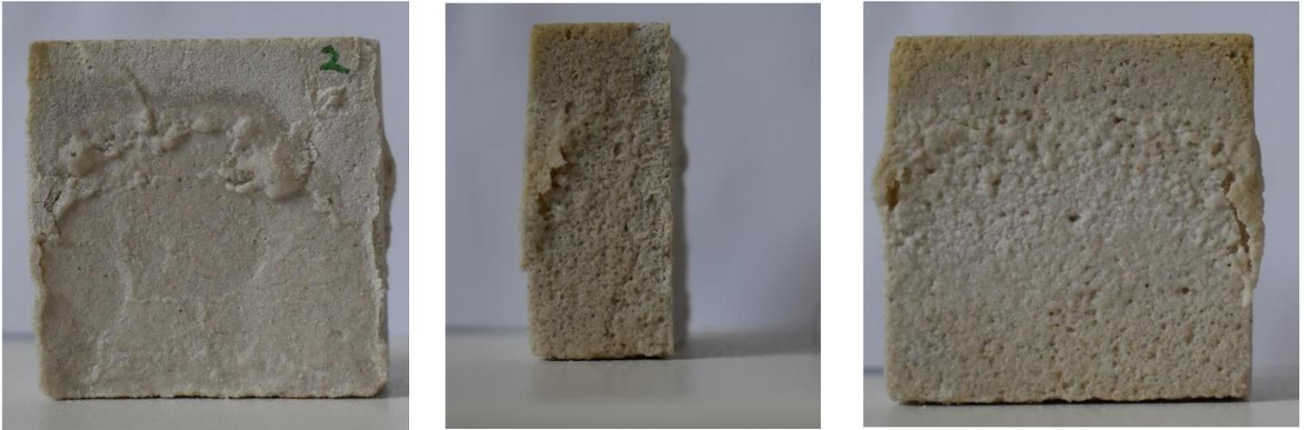
Figure 31: Visible detachment on the TQ-HL samples after the 5th cycle of the salt crystallisation test
