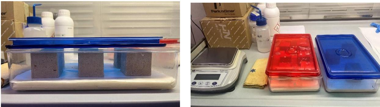
Figure 15: Set up for water absorption by capillarity test
