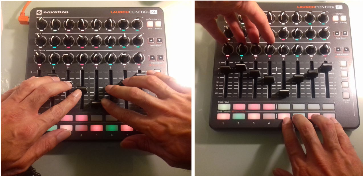
(a) left-hand fingers on faders 1–4 (control group 1); right-hand fingers on faders 5–8 (control group 2);
