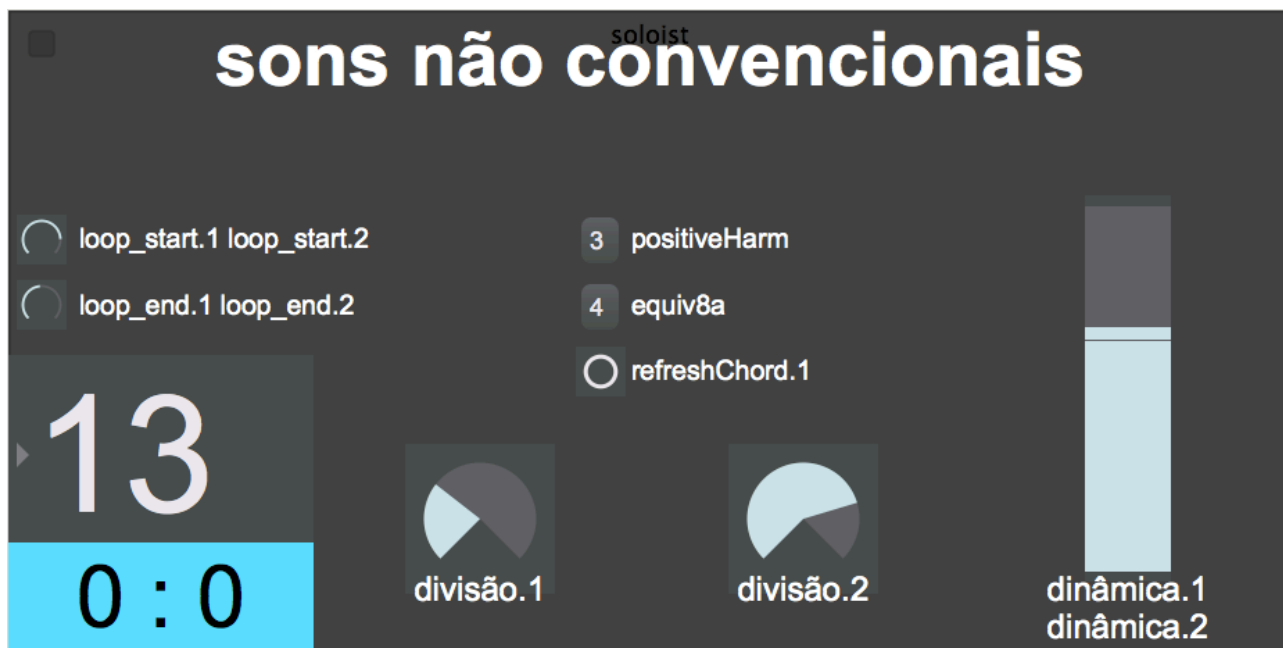
Figure 5.4: A miraweb-enabled visualisation interface for HASGS controller feedback and Comprovisador messaging. Messages from the host are displayed at the top. The parameter names assigned to each controller are subject to remapping upon preset change. The preset number and timer can be viewed at the bottom left.
