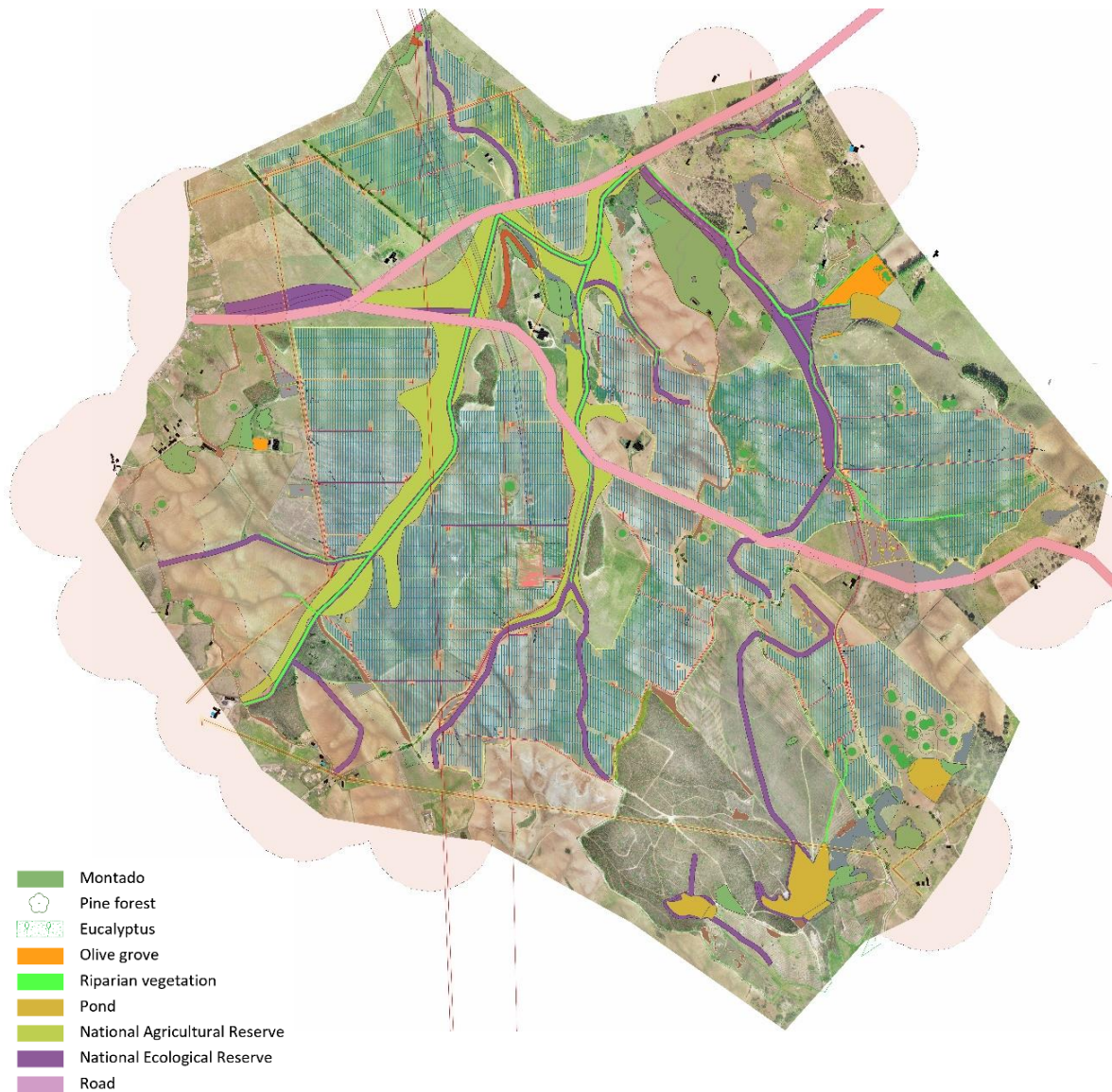
Figure 3.11: Environmental constraints at the Cercal Power PV plant implementation area identified through the environmental impact assessment [144].
