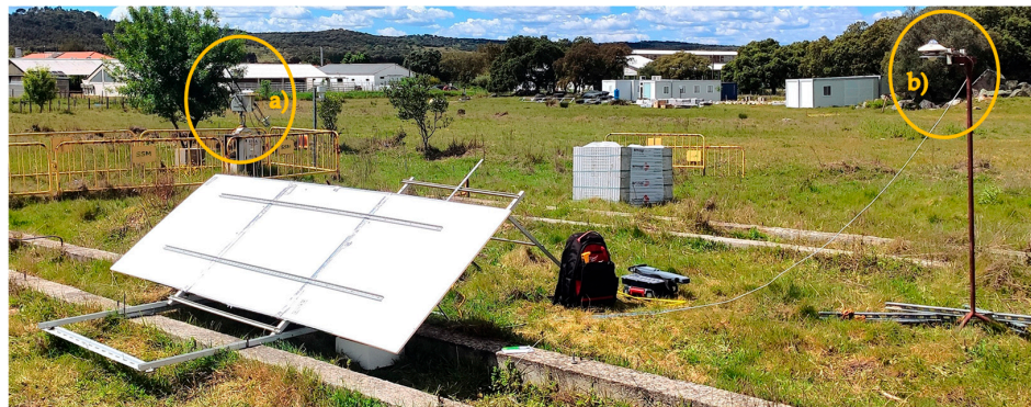
Figure 4. Overview of the experimental setup including (a) the Évora-PECS station and (b) the pyranometers used for albedo computations.
