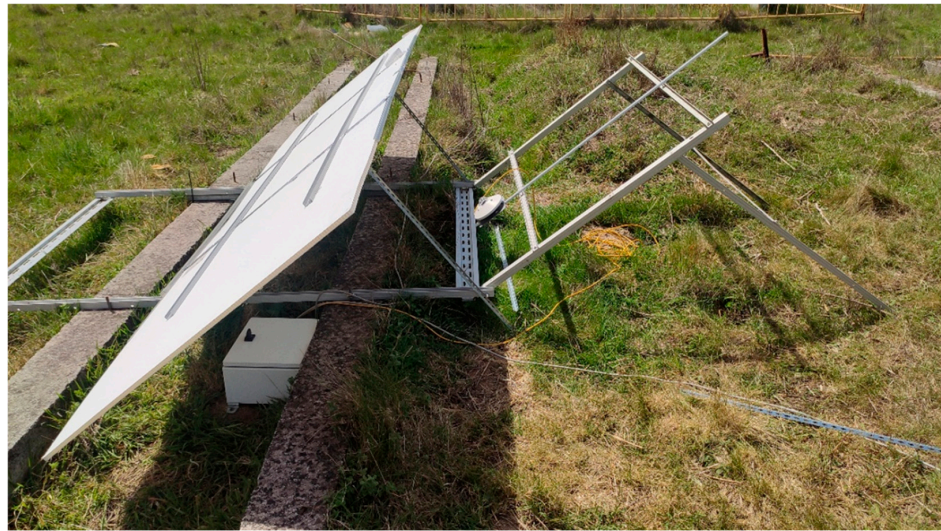
Figure 3. Experimental setup for measuring global tilt irradiance for different positions.
