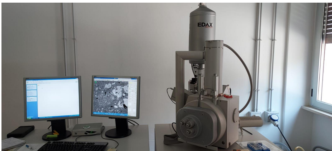
Figure 34. FEI Quanta 400 scanning electron microscope with attached EDS detector (Department of Earth Sciences, Sapienza University of Rome).
