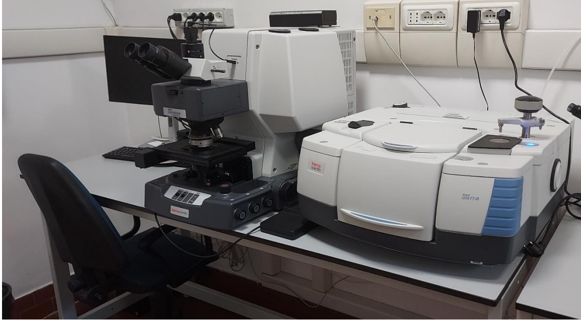
Figure 37. Nicolet iS50 FTIR Spectrometer paired with Nicolet Continuum IR Microscope from Thermo Scientific and OMNIC software for Windows 10 (Department of Earth Sciences, Sapienza University of Rome).
