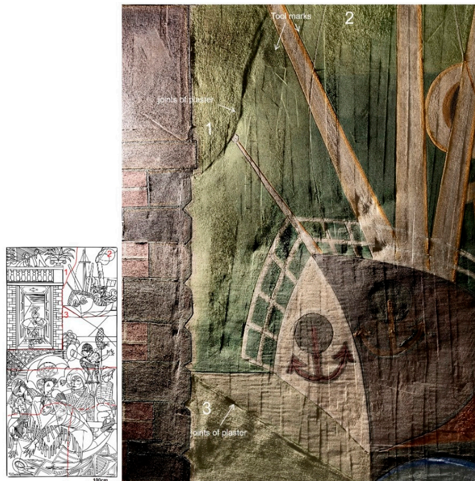
Figure 3. On the left, location of the plaster patches observed in mural P1. Patch n°2 is in the top left corner. On the right, details in Vis-Rak of patch n°2 and adjacent areas of patches n°1 and n°3, showing the intense presence of tool marks on the former when compared to the surface of the other two. The marks were made by repeated pressure movements exerted vertically, presumably after the painting was done, as evidenced by the differences in the texture of the paint on the green background and on the mast of the boat (photo by M. Ribeiro, drawing by K. Rix 2022).
