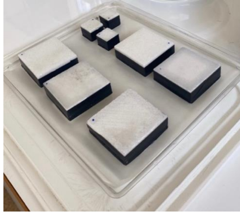
Figure 13: Optimization run to test water absorption by capillarity
