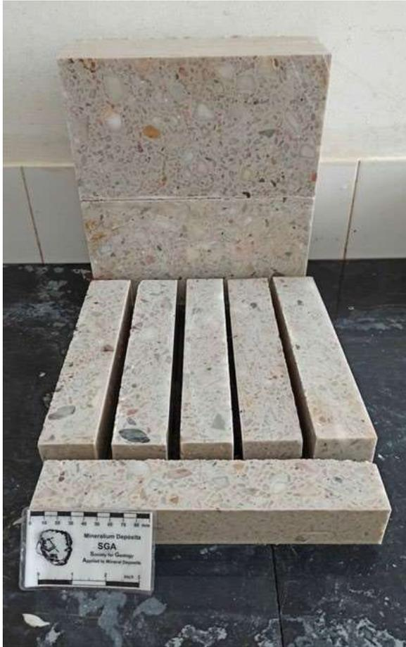
Fig. 7 Specimens obtained from cutting the block with a marble sludge binder.
