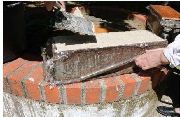
Fig. 6 Stone composites formulation mixing and vibration in the mold.
