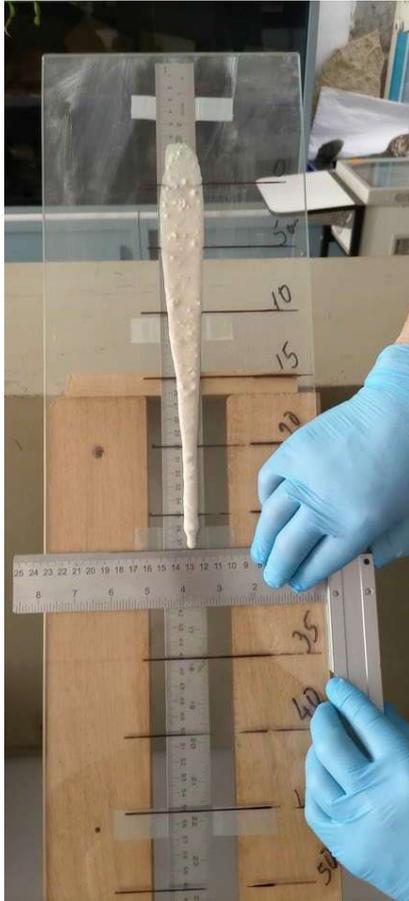
Fig. 4 Experimental set-up for viscosity and rheological measurements
