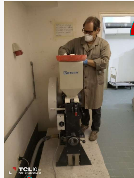
Mechanical disaggregation in jaw mill
