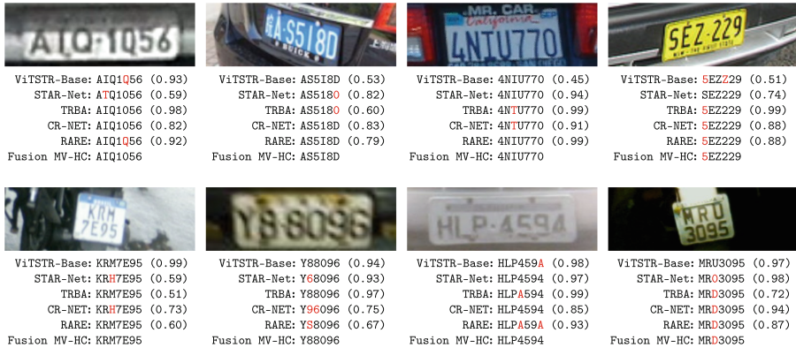
Fig. 4. Predictions obtained in eight LP images by multiple models individually and through the best fusion approach. Although we only show the predictions from the top 5 models for better viewing, it is noteworthy that in these particular cases, fusing the top 8 models (the optimal configuration) yielded identical predictions. The confidence for each prediction is indicated in parentheses, and any errors are highlighted in red. (Color figure online)
