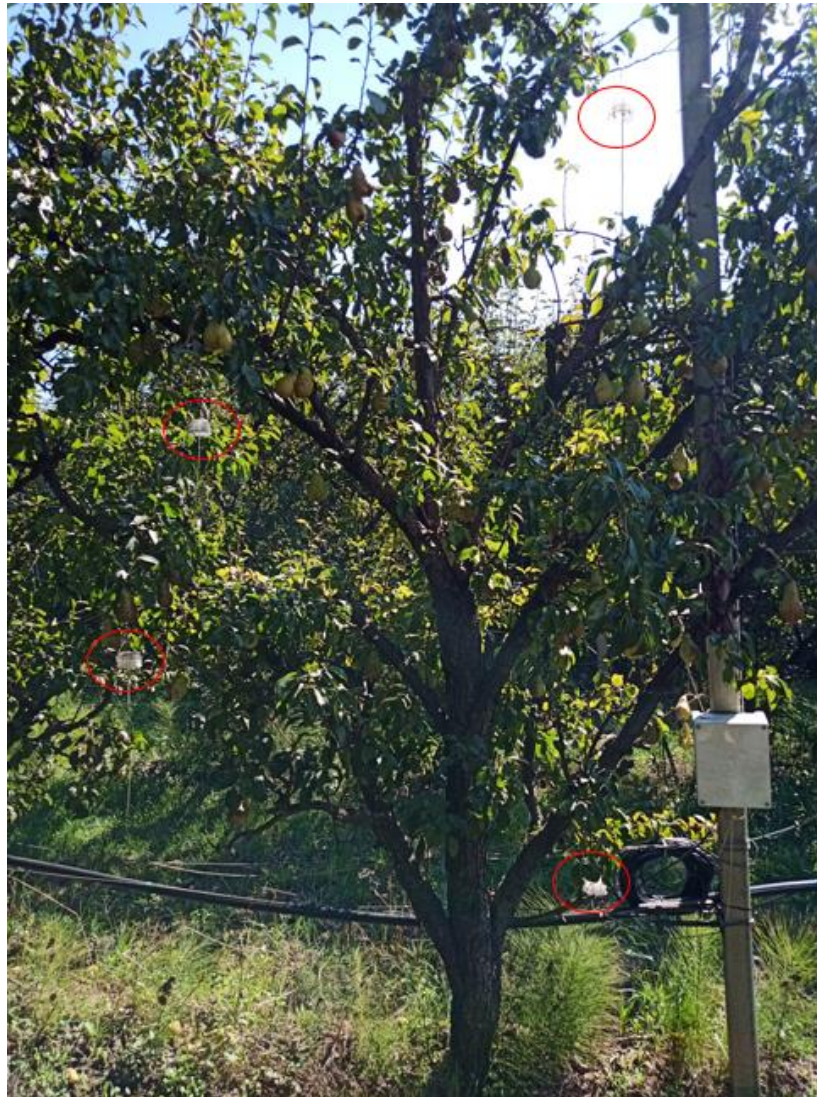
Figure 3. 6 - Different sensor heights on trees in the Haly.Id experimental orchard in the red circles in the pear tree
