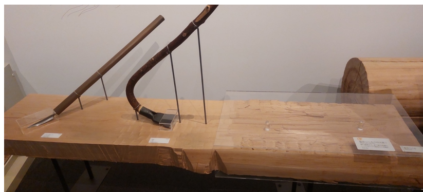
Figure 97 Tools displayed in the position of use. The wood shows the marks the instruments create in its surfaces. As these are instruments with sharp blades, the cutting edges were protected with acrylic cases. Photo: author.
