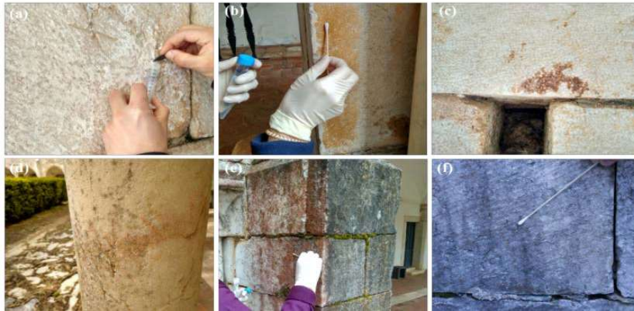
Figure 1. Main pathologies present in the Convent. Formation of white (SJP1) and yellow (SJP2) patinas (a, b), red stains (SJP3 and SJP4) (c, d), and formation of red (SJP5) and blackish (SJP6) biofilms (e, f).
