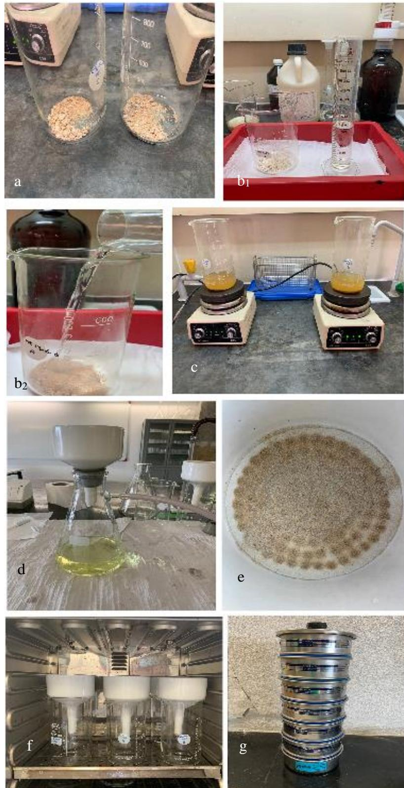
Figure 3.6 Experimentation of the analysis: a) sets of 2 samples, b1,2) HCl aqueous solution and the analyzed sample, c) Heating up the sample in HCl aqueous solution to boiling temperature, d) Filtration under vacuum using a Büchner funnel, e) Filtered wet sample using filter paper, f) samples in the oven to dry, g) Sieving using ASTM E11 test sieves.
