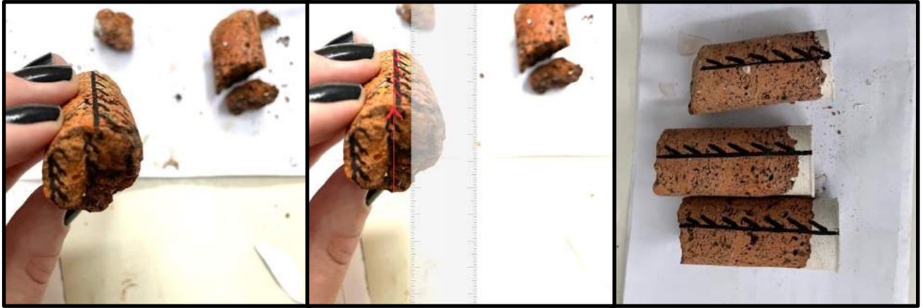
Figure 38. Images showing the laboratory arrow (x-axis) on the surface of the cores and transcribed down the length of the cores after drilling. It is important to follow the direction of the laboratory arrow on the top surface so that the orientation has the right position and direction down the length of the core.
