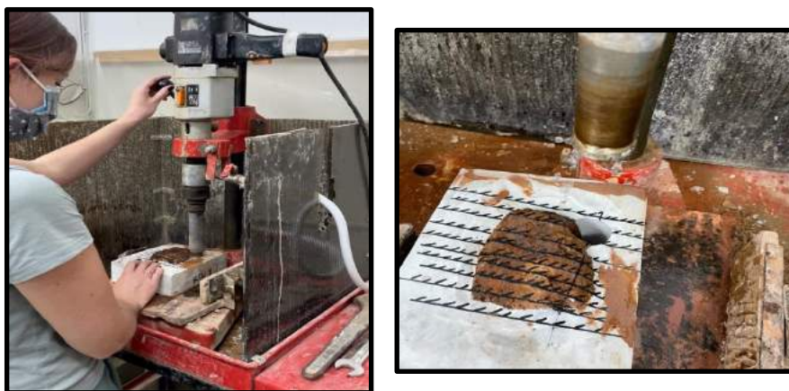
Figure 37. Drilling the cores. Using a diamond core drill, the cores were drilled perpendicular to the oriented surface. This process is time consuming as the slower the cores are drilled the less chance there is that the cores will be broken during this process.
