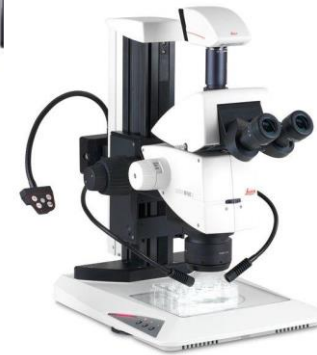
(g) A Leica M205C stereo microscope, used to observe the inclusion in the core of the crucible fragments
