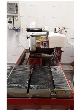
(h) An electric saw, used for cutting a small part from the slag samples for the EDXRF analysis
