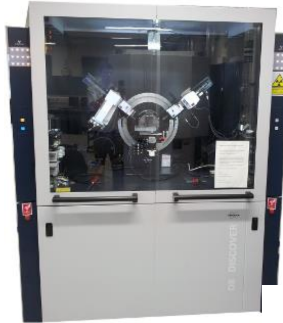
(b) A Brucker D8 Discover Diffractometer used for the powder XRD analysis
