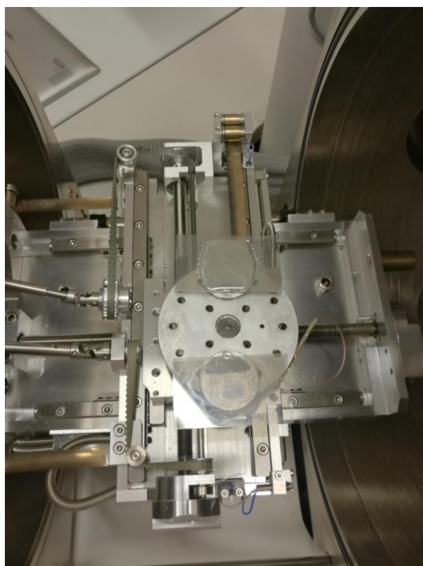
Figure 22 two sample in FEI Quanta 400 SEM (EDS) chamber
